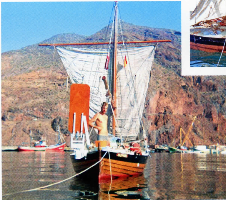
Left: a trial setting of the storm sail rigged upside down as a square sail in Santa Cruz harbour, Tenerife, Canary Islands
