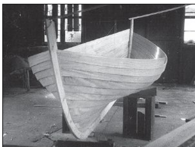
Tom Edwardson built AEGRE in 1966 using 11, 1/2"-thick mahogany planks per side. The sheerstrakes were larch, and fastenings copper.
